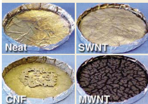
The residue of poly(methyl methacrylate) with various nanoadditives after heating.
